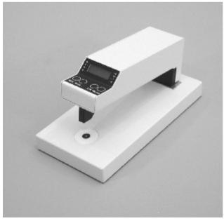
Heiland densitometers are build in a solid metal box and are powered by 12VDC by means of a wall plug power supply, that is included in delivery. The densitometer consists of the base unit and the measurement arm (lever). Both parts are connected via a precise bearing, the integrated spring pushes the arm in the upper position after releasing. The probe is mounted underneath the lever.
